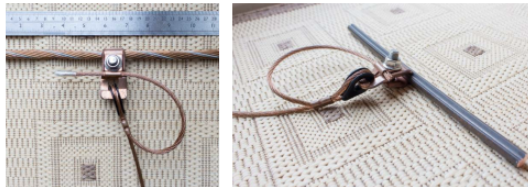
Figure 206 (l-r): Arthur Flury Bz II flexible current carrying dropper with CuNiSi clamps; catenary attachment and contact wire attachment
